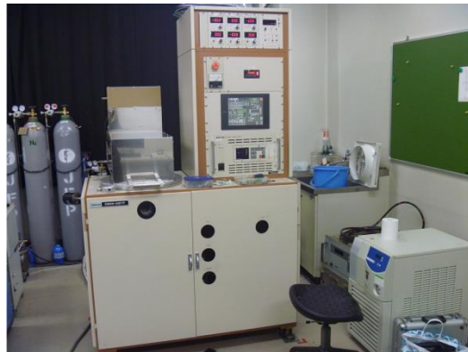
Fig.2: ICP dry-etching machine. The designed devices are fabricated using this equipment.
