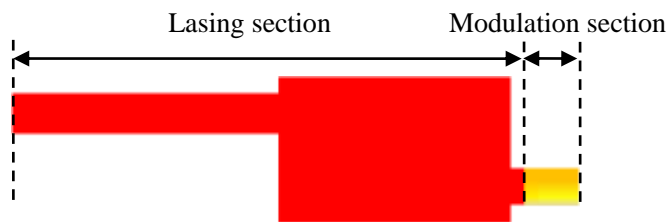
Fig. 1. Schematic of asymmetric active MMI LD
